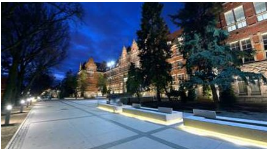
Concrete, backlit seats with a granite-like cover, along the illuminated zone (Source: U-Mob Project, 2018)
